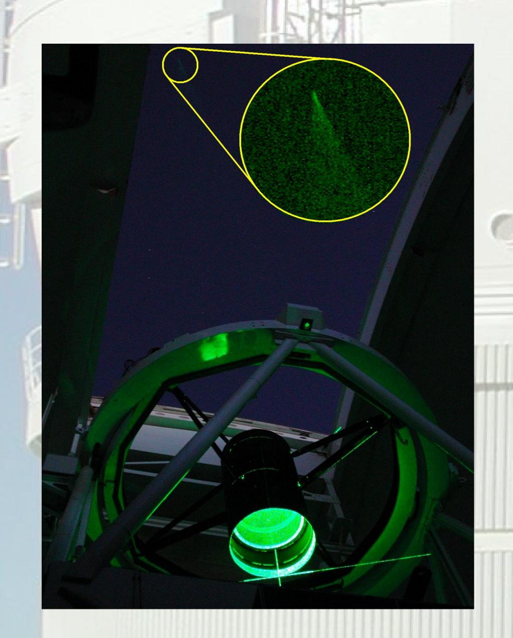
These two images show the high power laser launch through the 30cm f/6 launch system (above) and the WHT (left). Safety considerations form a major part of the project. The laser is only operated by trained staff using protective goggles to prevent eye damage. A plane spotter is used to ensure that no harm comes to aircraft that may fly through the laser beam (the mountain top itself is actually a 'no fly' zone).
