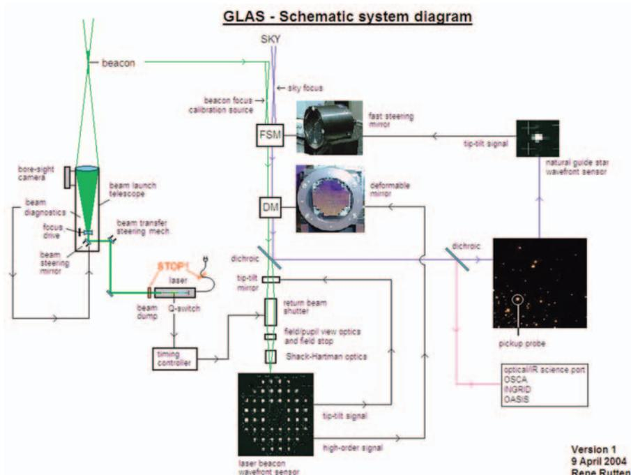
Figure 2. System diagram for the GLAS and NAOMI system.
