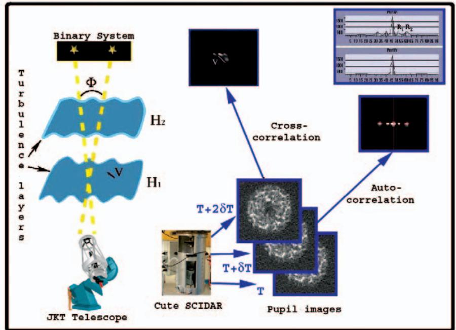
Figure 1. SCIDAR technique layout. From the observation of binary stars, we get a stack of consecutive images of scintillation. The average auto-correlation function of them gives information of the  $C_N^2$  profiles, and average cross-correlation functions give the wind of the layers.
