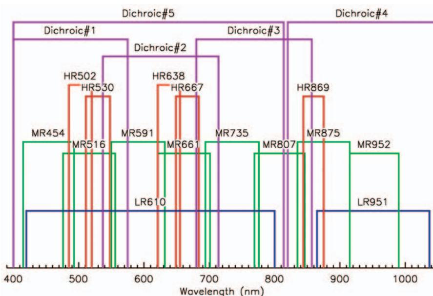
Figure 1. Spectral configurations of OASIS. Blue lines indicate the low-resolution (LR) modes ( $R \sim 1000$ ); green lines indicate medium-resolution (MR) modes ( $1000 < R < 2000$ ); and red lines indicate high-resolution (HR) modes ( $R > 2000$ ). The dichroics are required to isolate the science light from the NAOMI AO system.
