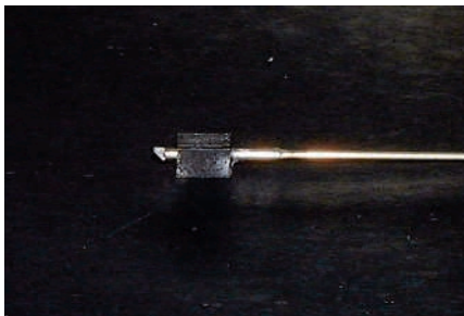
Figures 1 and 2: Top and side views of a fibre prism and gripper button.
