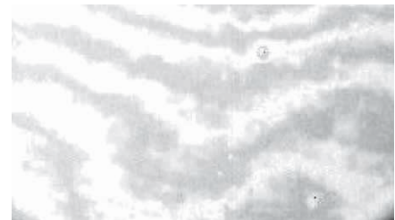
Figure 1. Image showing the effects of fringing in a thinned astronomical CCD.
