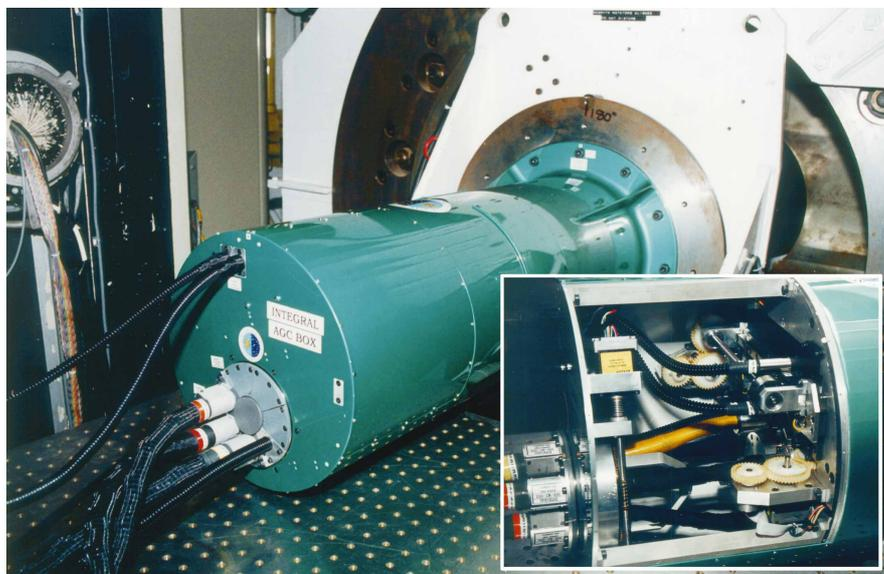
Figure 1. Acquisition, calibration and guiding structure of INTEGRAL.
