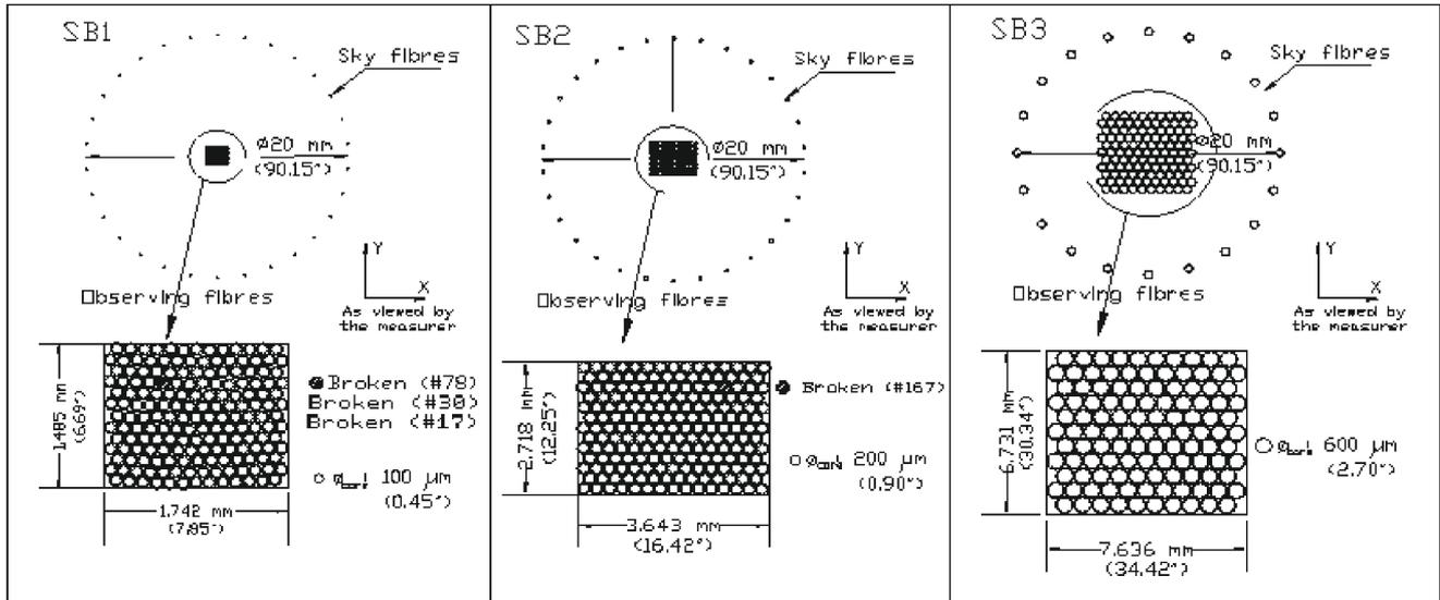
Figure 2. Configuration of the three standard bundles of INTEGRAL at the focal plane of the telescope. Note that the external ring of fibers is intended to collect the sky background simultaneously to the object observations.
