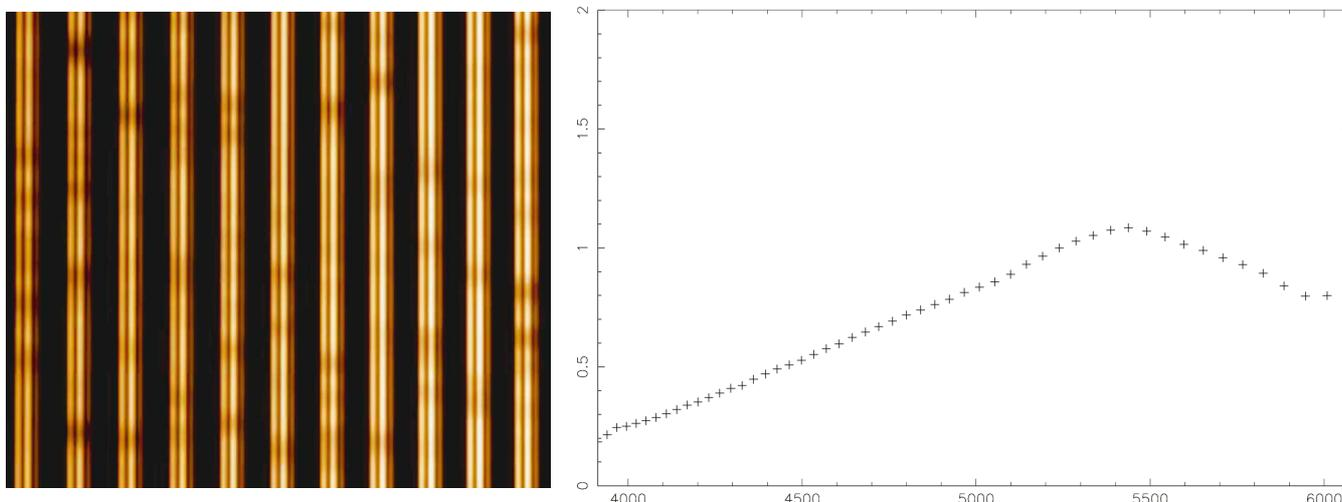
Figure 1 (left). This shows part of a UES exposure of  $\tau$  Boo obtained with the fibre feed — the orders appear striated because of small gaps between the three slices from the input fibre. Figure 2 (right). The average relative transmission for different Echelle orders between an exposure taken with the fibre, and one taken through the de-rotator (see text for full description). These are plotted as function of wavelength in Angstroms.
