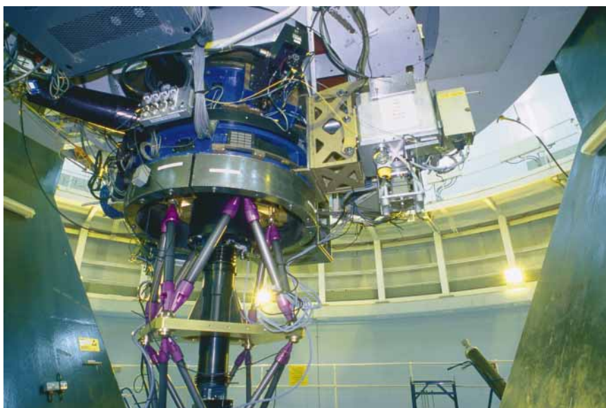
Figure 3. INGRID mounted on one of the WHT folded Cassegrain foci (top right). The instrument on the Cassegrain focus is SAURON. Picture credit: Rainer Girnstein.
