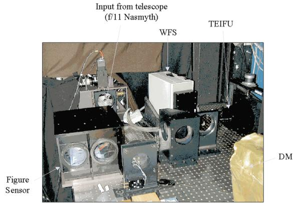
Figure 2. Schematic layout of ELECTRA at GHRIL (WHT).
