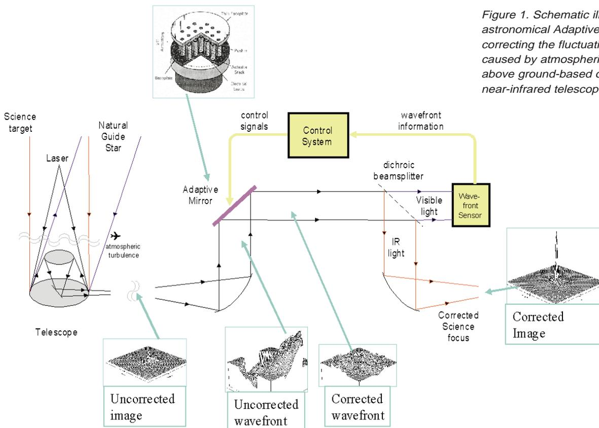
Figure 1. Schematic illustration of astronomical Adaptive Optics for correcting the fluctuating aberrations caused by atmospheric turbulence above ground-based optical and near-infrared telescopes.
