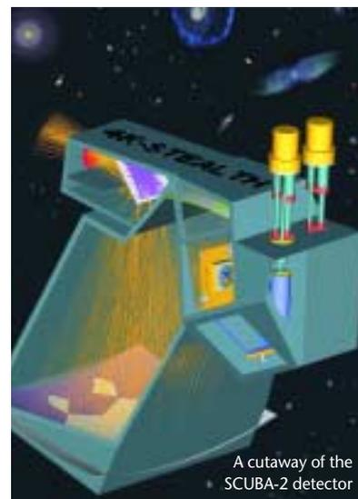
A cutaway of the SCUBA-2 detector
