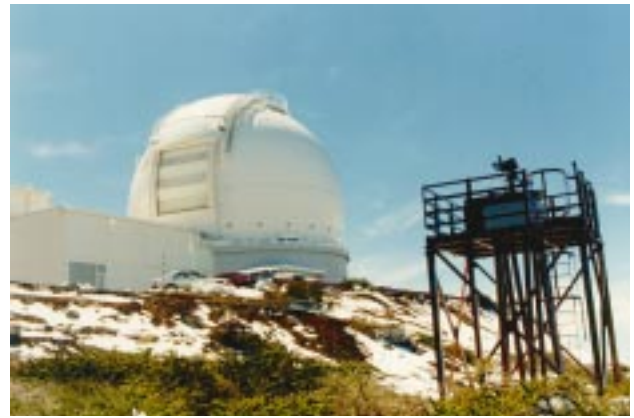
The tower with the DIMM on the top at a height of 5 m above ground. The DIMM is based on a 20 cm Celestron telescope. The WHT in the background is 50 m away and about 15 m above the level of the DIMM.
