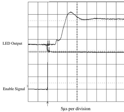
*Figure 4) Switch-on delay of lamp*
