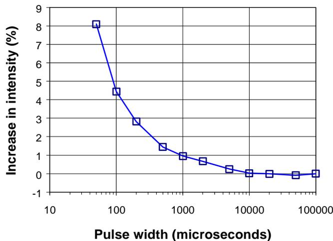
*Figure 6) Intensity of lamp as a function of switch-on duration.*
