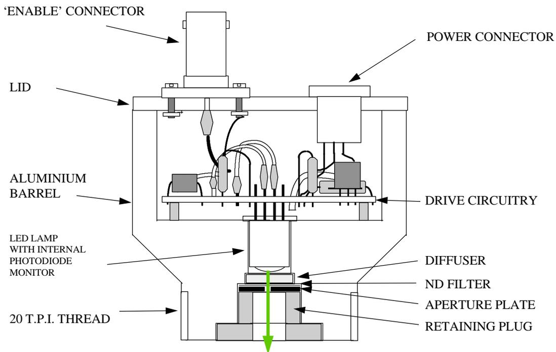
Figure 2) Schematic of the Linearity Lamp
