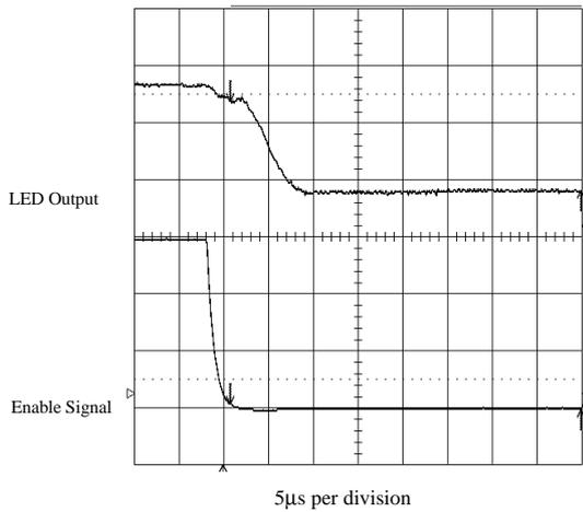
*Figure 5) Switch-off delay of lamp*
