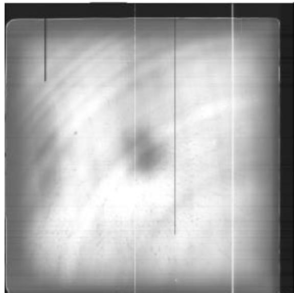
*Figure 11) A Flat field image from a recently UV flooded Loral Lick 3 CCD*
