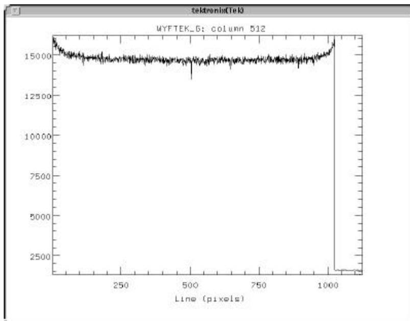
The flat field projector was also used to diagnose QE degradation due to surface contamination in a Loral Lick 3 CCD. Figures 10 and 11 show flat field images taken before and after UV flooding. It is easy to see that the QE has been degraded in the first image even without making accurate QE measurements.
