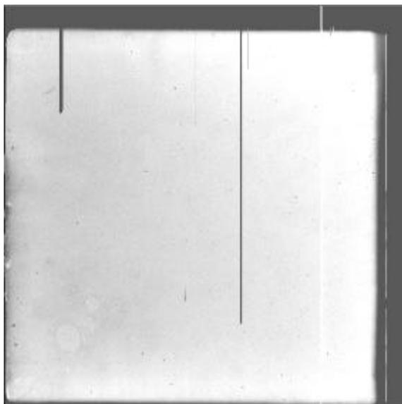
The flat field projector has also been used with the new large format EEV42 CCDs. The spreadsheet model predicts a 4.5% drop-off in illumination at the corners of this larger (28 x 55mm) device. Nevertheless the flat field images obtained, one of which is shown in figure 12, are still very useful.
