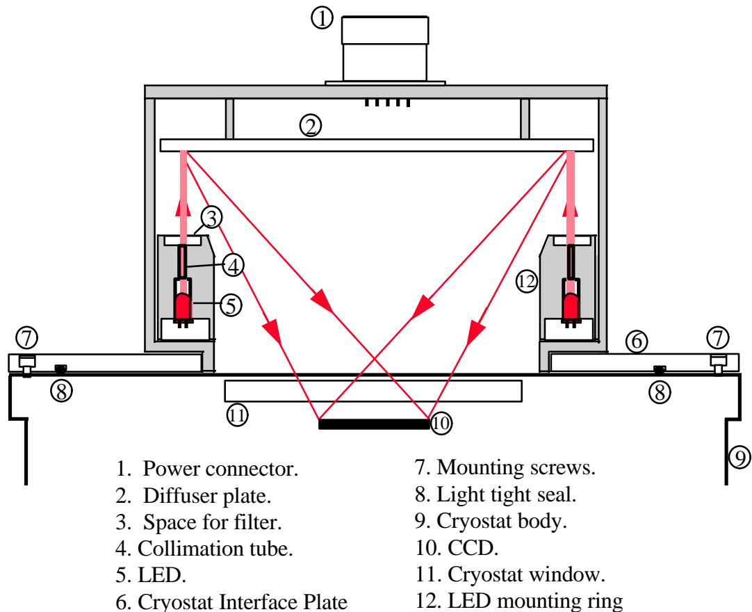
**Figure 6) Detail of LED Mounting Ring.**
