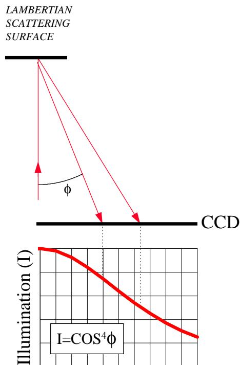
Clearly a single Lambertian scattering source will not by itself provide a flat field illumination.
