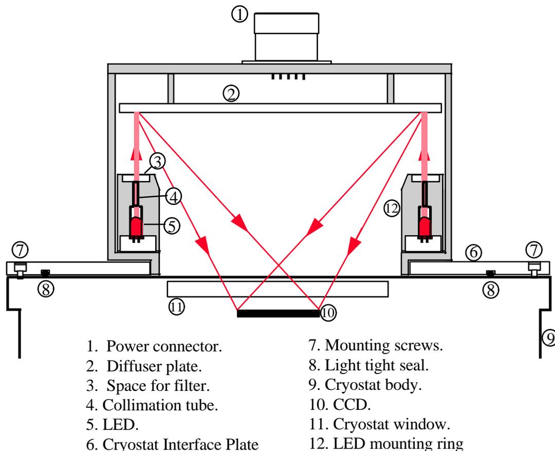
Figure 6) Detail of LED Mounting Ring.
