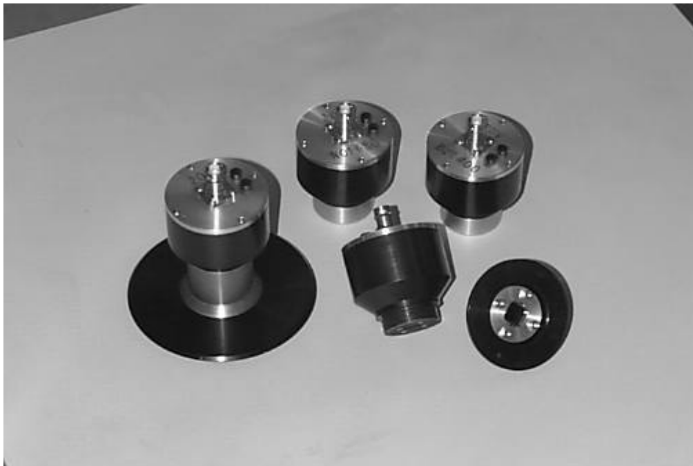
Figure 1) Four of the light sources with a calibration photodiode at bottom right.
