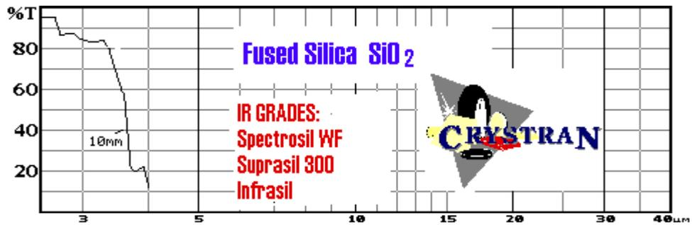
Figure 2.3 Optical Transmission of focal plane mask substrates
