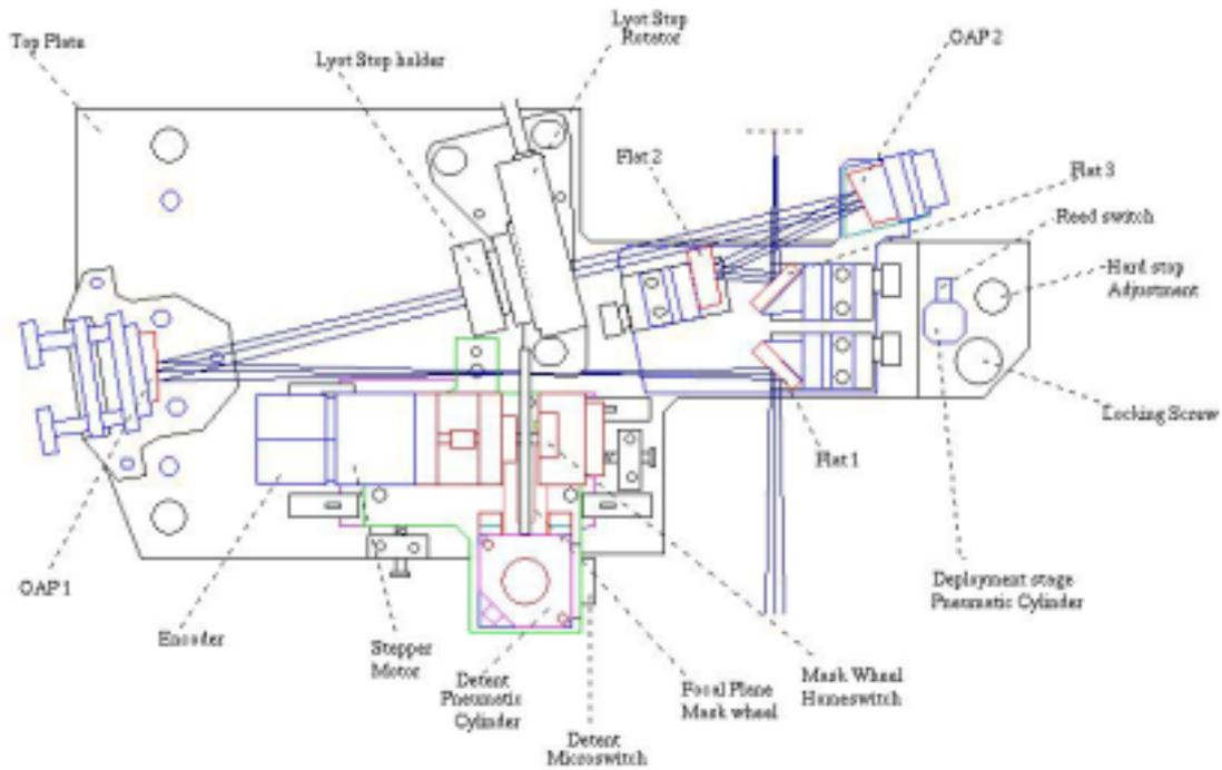
**Figure 3.1 Schematic top view of the OSCA unit**
