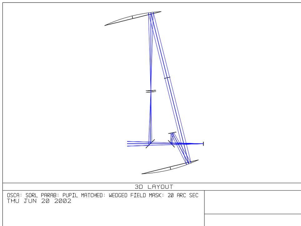
**Figure 2.1 Zemax optical design of the OSCA system**
