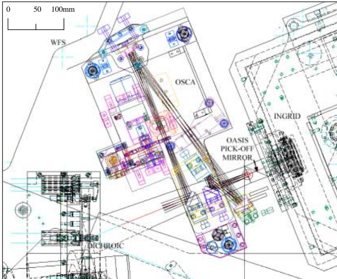
**Figure 1.1 OSCA unit relative to the other components on the NAOMI optical table in GHRIL.**
