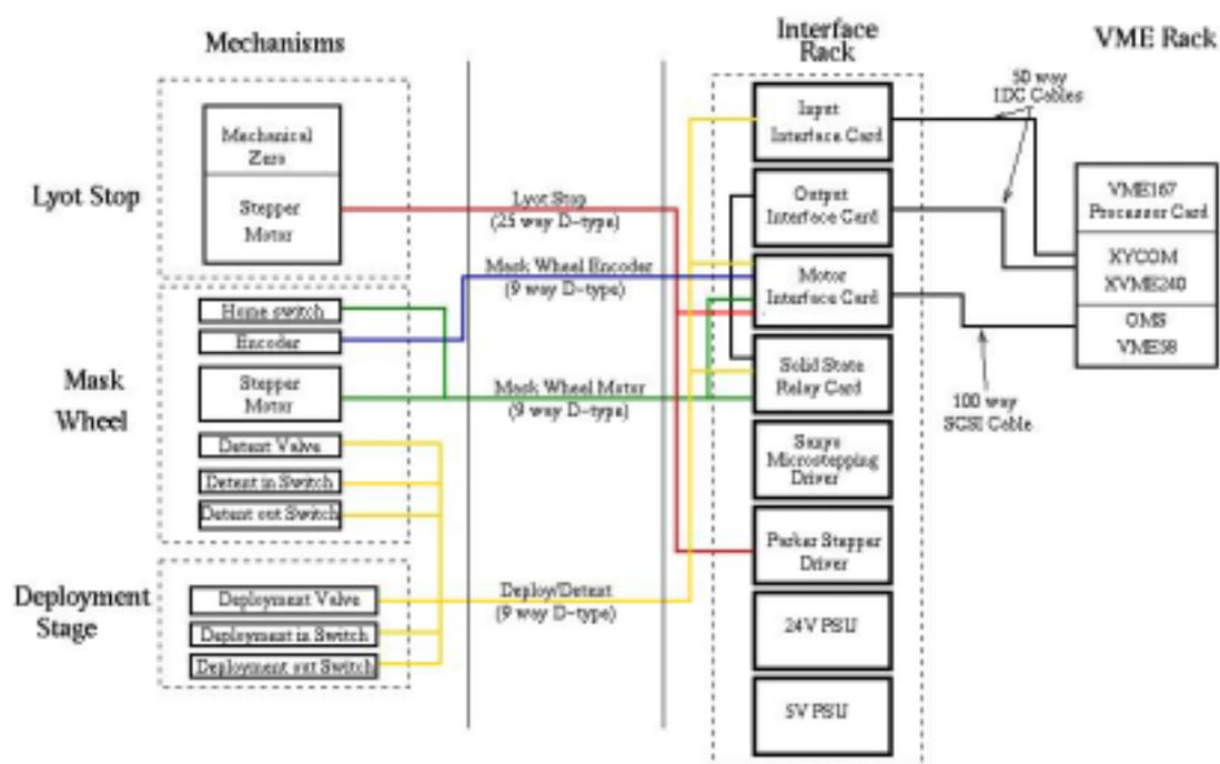
Figure 4.1 Schematic of OSCA electronics
