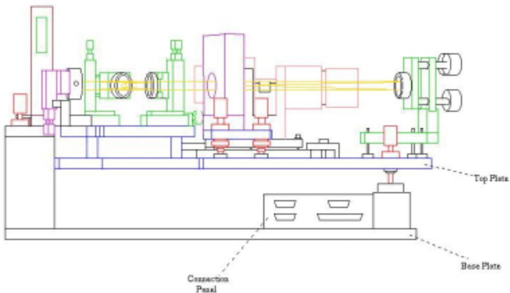
**Figure 3.2 Schematic side view of the OSCA unit**
