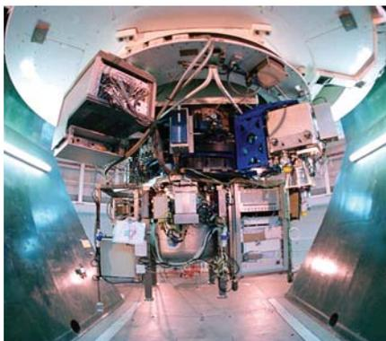
Figure 1 (top left). LIRIS mounted on the WHT Cassegrain focus. LIRIS cryostat can be seen at the bottom of the telescope focus, with the two electronics racks at both sides. Figure 2 (top right). The globular cluster M5 in the *J* band. The FWHM of the PSF was 2 pixels corresponding to 0.5". The image quality is very good over the whole field of view (4.2 arcmin<sup>2</sup>). Figure 3 (right). Arrival of LIRIS at the WHT in January.
