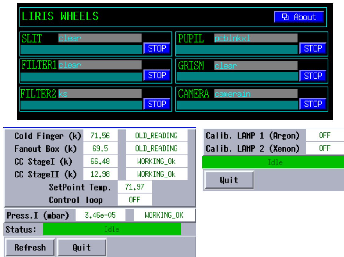
Figure 3.6: The LIRIS status mimics. Top: the current filter/slit/grism configuration; lower left: the temperature display (window looks a bit different nowadays); lower right: the status of the two arc lamps
