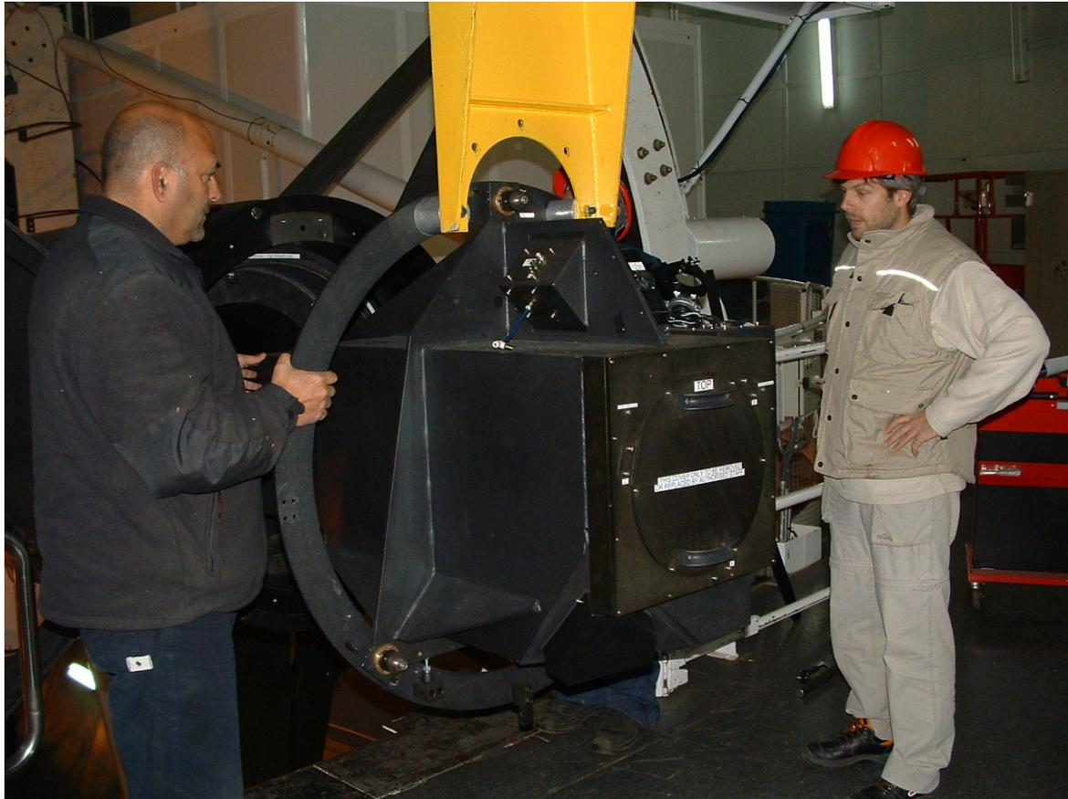
13. Using the 2.5 ton dome crane attach the yellow lifting frame to the BLT and tension the crane to take the weight off the BLT.
