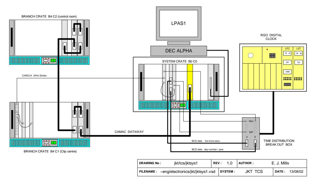
Figure 1 JKT CAMAC Crate layout, dataway and Time Service cables
