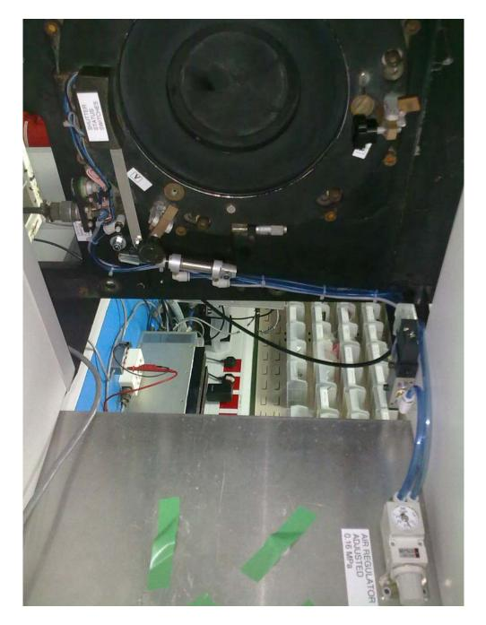
With this modification a new air flow control for the ventilation of the window of the cryostat has been installed.
