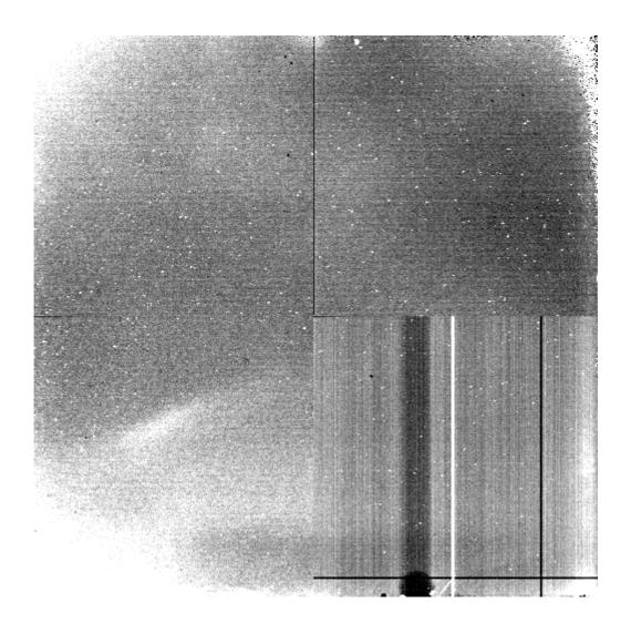
HAWAII Engineering array Mean Bias image – mean of several images Taken using old IRLabs Preamp and fanout board Different radiation leakage to image seen above !!! Note cross talk ghost images of "hot" column
