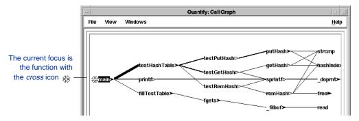
To change the focus of the call graph to a new function, right-click the desired function and select **Change focus > Focus on subtree** from the pop-up menu.
