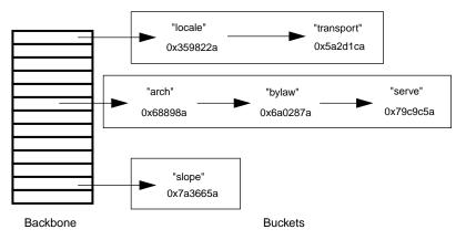
Given a string token such as "serve", the hashtable package computes a 32-bit hash key, in this case 0x79c9c5a, based on the characters in the string. The hashtable package uses the hashkey *modulo* the size of the hashtable backbone to determine what bucket to search and then scans the entries in the bucket looking for the entry with the same string. Here is the source code for the testHash program.
