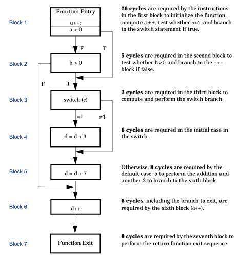
To execute the first call to test(0, 1, 3, 8) in main, the program enters blocks 1, 3, 5, 6 and 7, which takes 51 cycles. The table below compares the difference in cycle counts between optimized and non-optimized code. The optimized version is noticeably faster, primarily because all the calculation occurs in registers, thereby avoiding the need to load and store values from memory.
