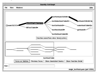
The functions that are called after the call to testPutHash are also recorded, even though these functions contribute no time.
