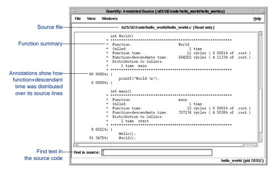
The numeric annotations in the margin reflect the time recorded for that line or basic block over all calls to the function. By default, Quantify shows the function time for each line, scaled as a percentage of the total function time accumulated by the function.
