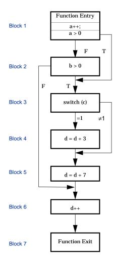
Here is the basic block flow structure of the test function:
