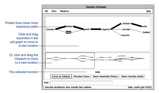
By default, Quantify expands the call paths of the top 20 functions that contribute most to the overall time of the program. The call graph begins at the .root. accumulator, which represents the total amount of time used by all the functions in the program. For more information about the .root. accumulator, see "How Quantify records function time" on page 3-2.
