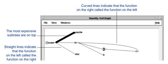
If a function is not a leaf function, a triangle indicates how many of each function's immediate descendants are shown in the call graph.
